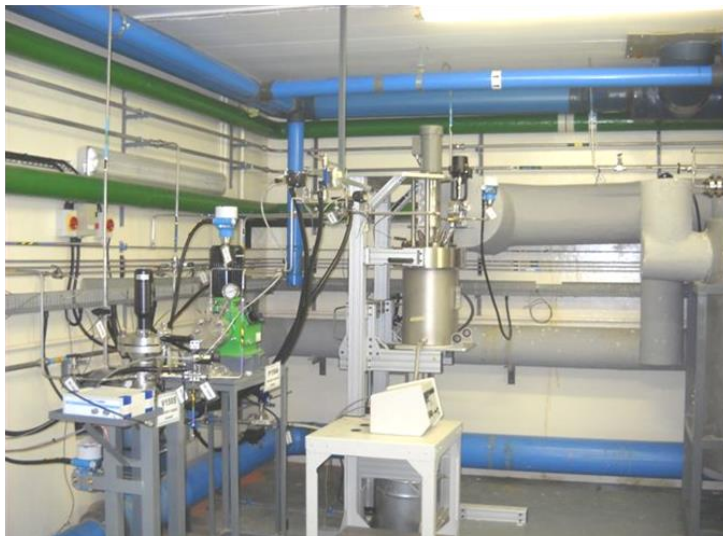
Polymerization reactor and initiator feed system showing dosing pump
